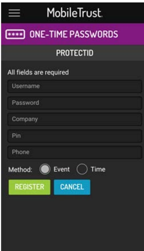
After inputting the necessary information and tapping the "Register" button, the app will register and synchronize the OTP generator with the users profile on the ProtectID server
