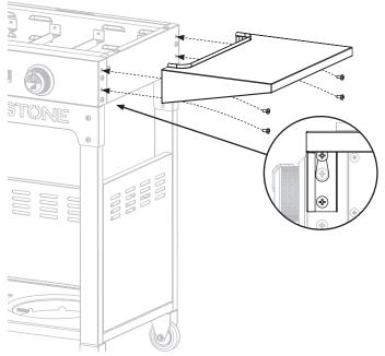
**STEP 13** Use four (4) of the removed M6x12 bolts to secure one (1) side shelf to the left side of the griddle body.
