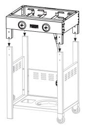
**STEP 04** With the help of another person, use two (2) M6x12 bolts [b.] to attach the left leg assembly to the left side of the cart base. (**Note:** loosely install both screws then tighten.)
