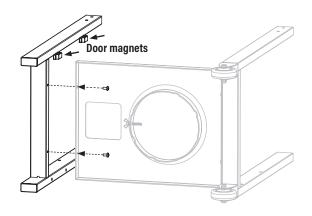
**STEP 06** Use eight (8) M6x12 bolts [**b.**] to attach the two (2) side panels to the left and right leg assemblies. DO NOT fully tighten the bolts at this time.
