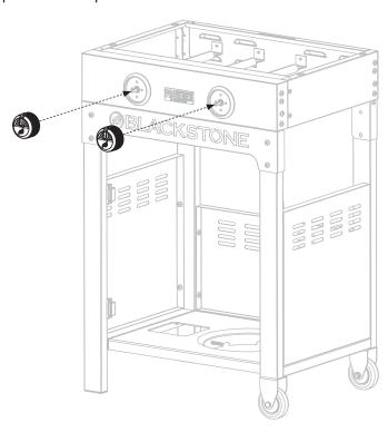
**STEP 11** Remove the top, and second-from-the-bottom eight (8) M6x12 bolts on either side of the griddle body.
