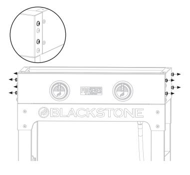
**STEP 12** Use four (4) of the removed M6x12 bolts to secure one (1) side shelf to the right side of the griddle body.
