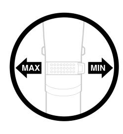
**3** Suction Control is located on handle. To decrease suction and reduce resistance, slide toward MIN. Slide toward MAX to increase.
