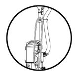
Use cord clip located on the side of wand to hold cord in place while vacuuming.
