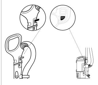
1 To clean with handle only, press latch to remove.
