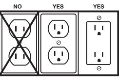
Two Prong **Three Prong Three Prong** non-grounded grounded grounded
