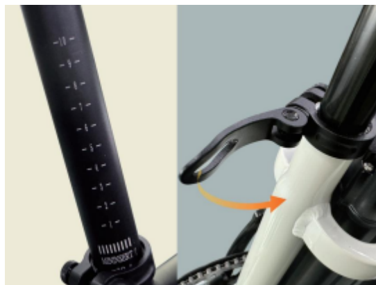
b. Adjust the height to your liking, and lock the latch.
