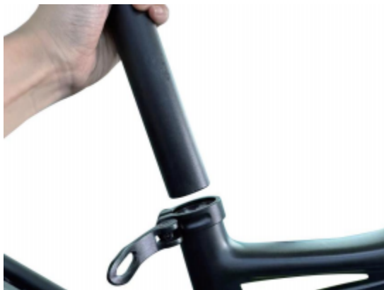
a. Insert the seat in the seat post.
