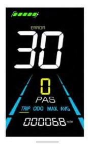
When one of these error codes appear on the display, kindly contact Mizari Customer Support for immediate assistance. The error is likely due to a communication problem between the controller and the display.
