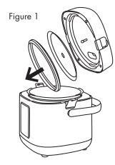
Remove Lid, Heat Shield and Silicone Ring for cleaning
