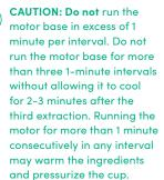
Friction from the rotating blade when extracting can cause ingredients to heat and generate internal pressure in the sealed vessel. If the vessel is warm to touch, allow to cool before carefully opening pointed away from your body.
